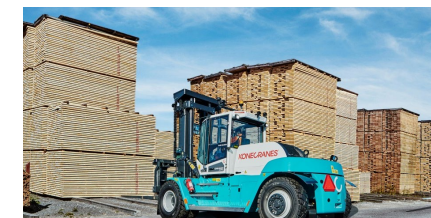
Fully-electric E-VER forklift (Li-ion)
