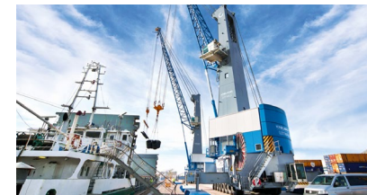
Fully-electric MHC (cable reel)
