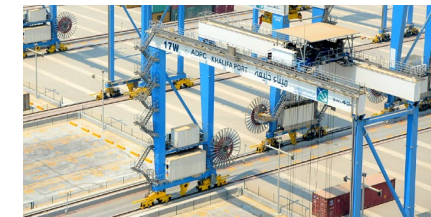
Fully-electric ASC/ARMG (cable reel)
